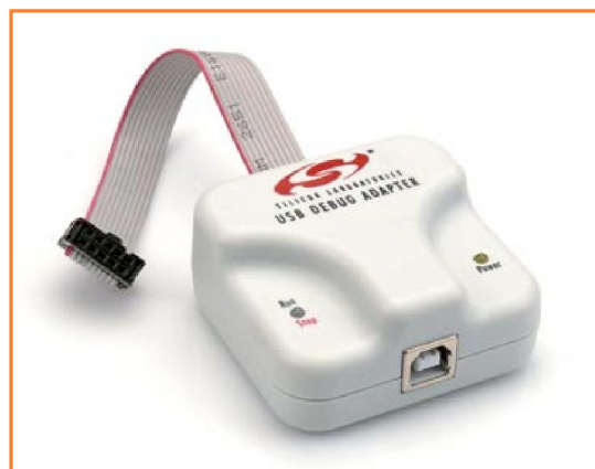
Figure 8. To load the program into a blank microcontroller, you'll need this accessory.
